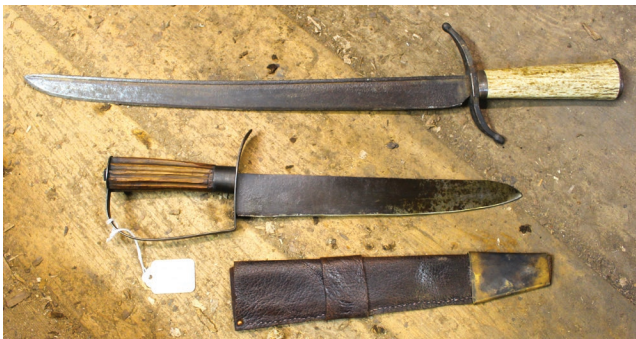
(top) Repurposed sword blade by Dan Aubhil. (bottom) Repurposed scythe blade and sheath by Ken Netting.
